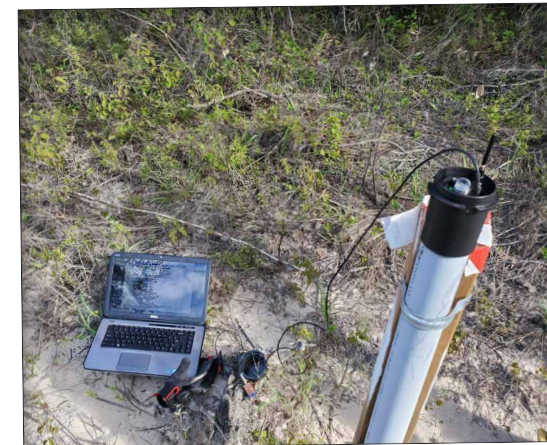
Downloading water level logger data and completing site maintenance.
