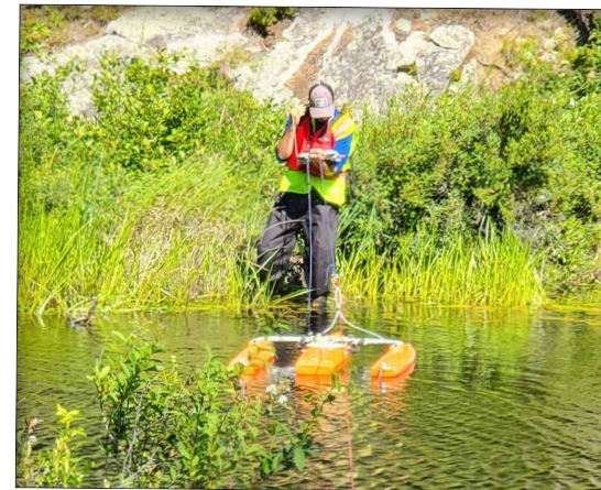
Stream flow measurement with a River Ray ADCP.
