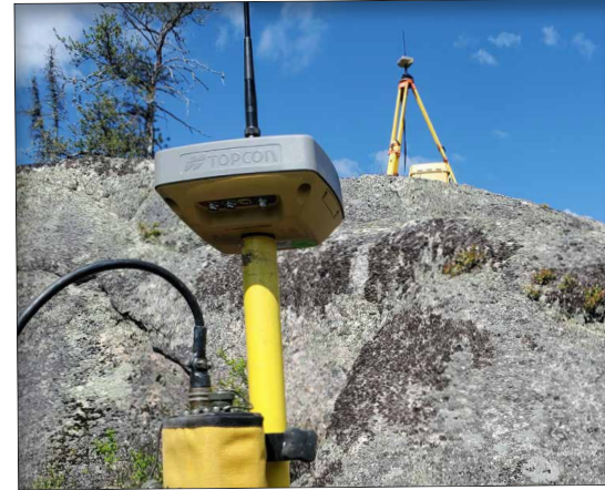
Base and rover setup to complete bathymetry survey.
